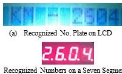
Fig. 19 – LCD & Seven Segments Displaying the Recognized Characters of the processed Number Plate
